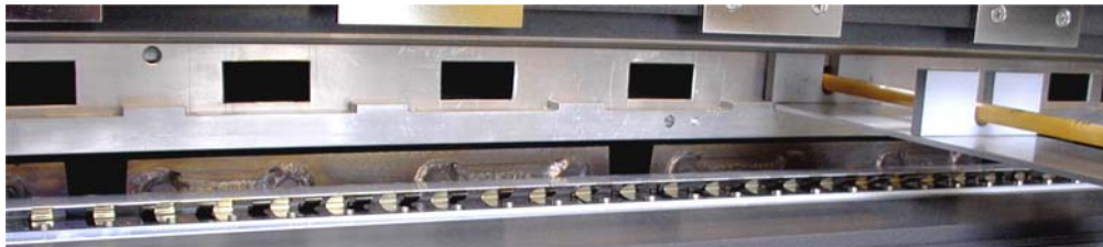
Fig. 4-6: Orifices in a metal plate contacting top and bottom plate of the KAI 1000 reactor. The shaft on the right side is the inserted E -field probe.
