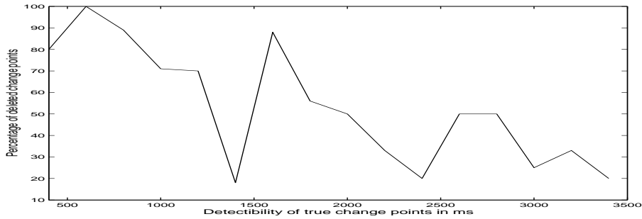
Figure 4.3. The histogram of deleted true reference speaker change points as a function of their detectability. The detectability of a speaker change point is defined as the duration of the segment following that change. The figure shows that the accuracy of the proposed algorithm depends on the detectability of true change points.
