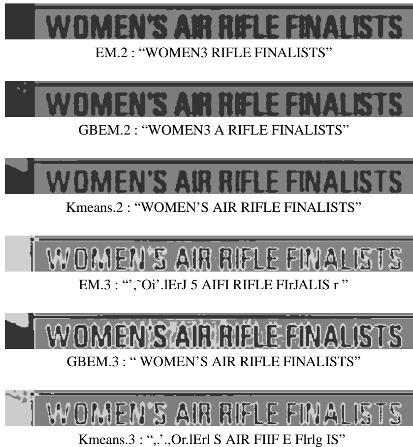
FIG. 5.13 – Segmentation output of the three studied algorithms and associated recognition results using 2 or 3 layers/classes.
