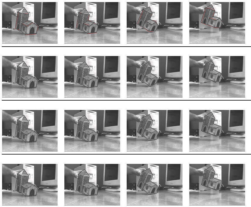
Figure 8: Comparison between different contour tracking algorithms. First row: Tracking results using our classifier based method and RANSAC. Second row: tracking results using an edge-based tracker. Third row: Tracking results using Fisher discriminant function. Fourth row: tracking results using texture boundary detection
