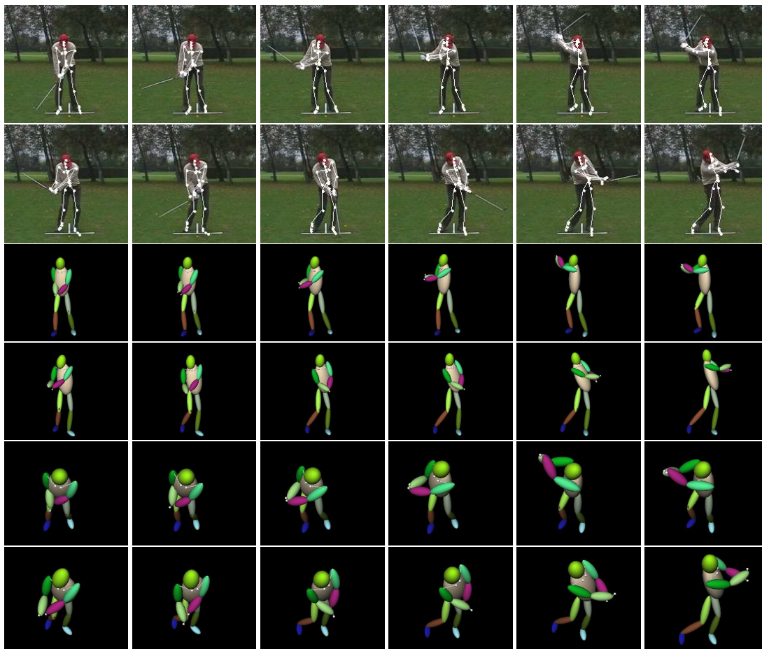
Figure 1: Tracking a full swing in a 45 frame sequence. First two rows: The skeleton of the recovered 3–D model is projected into a representative subset of images. Middle two rows: Volumetric primitives of the recovered 3–D model projected into the same views. Bottom two rows: Volumetric primitives of the 3–D model as seen from above.
