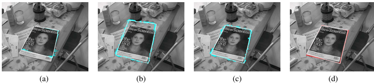
Figure 5. Frame # 90 for tracking using different methods: (a) edge-based tracker, (b) scanlines only, (c) scanstripes only, and (d) RANSAC linkage of scanstripes.
