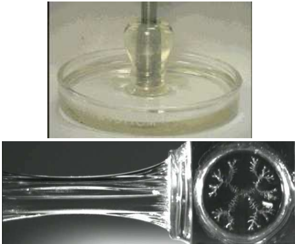
FIGURE 1. Top: Rod climbing effect or “Weissenberg effect”. A Rod is rotated with its end immersed in a viscoelastic fluid. Bottom: The separation of two plates with a thin layer of a viscoelastic liquid between them can lead to complex instabilities. For more details and original pictures see the web site of the group of Prof. Gareth McKinley at MIT HTTP://web.mit.edu/nmf/research/ . Reprinted with permission.
