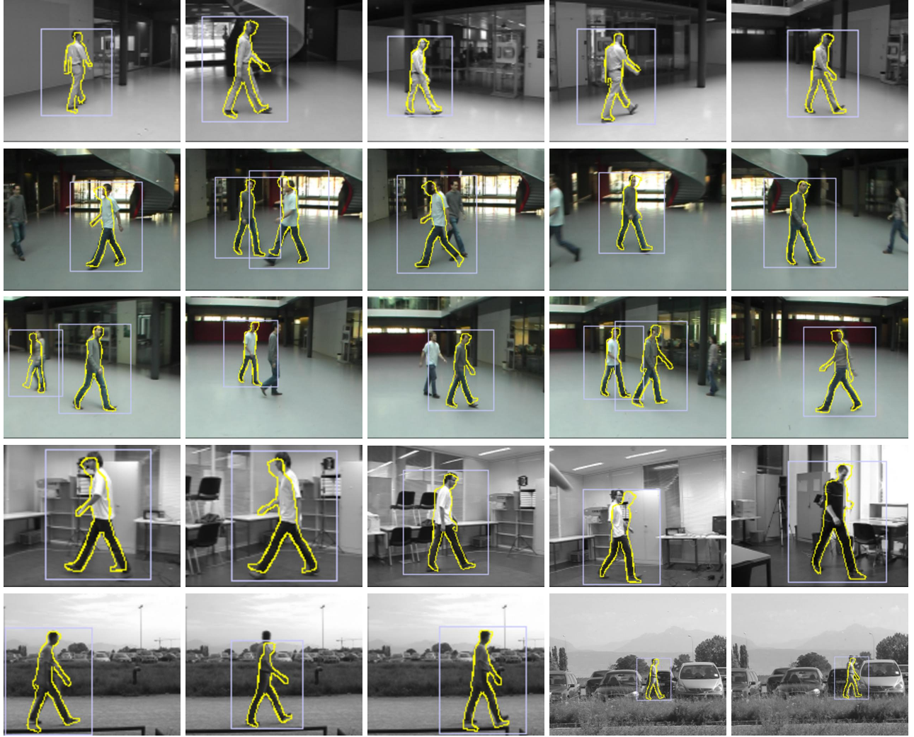
Figure 2: Detected silhouettes in several indoor and outdoor sequences acquired by a moving camera. Since we search for a specific posture —the one where both legs are on the ground and the angle between them is greatest— the fact that the algorithm does not respond to some of the people in the second and third image of the third row is correct. In that sense, the detection on the left of the first image in the third row is one of the rare false positives it produces. The sequence with several people is attached as a supplementary material.
