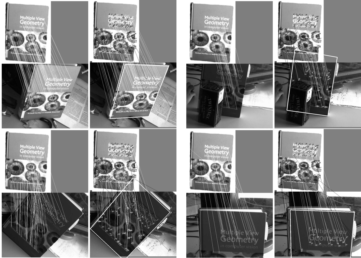
Figure 6: Comparison between SIFT method (left image) and ours (right) for a planar object. Our method usually gives a little less matches, and has a little higher outlier rate. Nevertheless, it is largely enough to accurately estimate the object pose after a few tens of RANSAC samples, with a lower computation cost than SIFT method.
