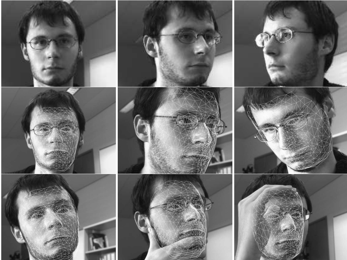
Figure 7: Face pose estimation. First row: the three training images for face pose estimation. They have been registered manually. The 3D model (not shown) is a generic human face model, and does not include the glasses of the subject. Second row: recovered pose under normal conditions. Third row: recovered pose under more difficult conditions. The subject removed his glasses in the first image, and the face is partially occluded in the two last images.
