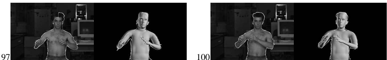
Figure 6: Applying the model-based silhouette extraction method of Section 5.2 to the sequence of Figure 3. The tracking errors around frame 100 have been corrected by combining stereo and silhouette information. The snake-optimized contours are overlaid on the original images and on the reconstructed body model.
