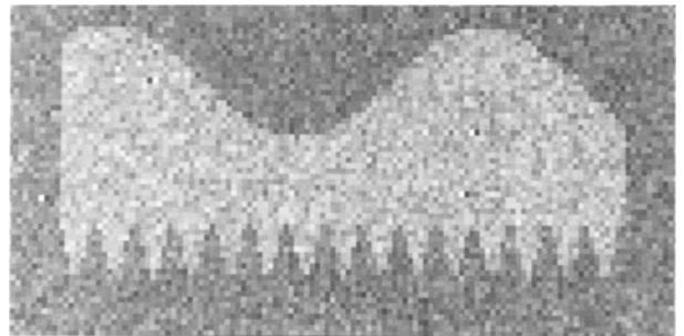
Figure 2. A synthetic image generated by adding white noise of variance 20 to a foreground with mean value 150 and a background with mean value 100. The lower and upper boundaries of the foreground are sinusoids of different frequencies.
