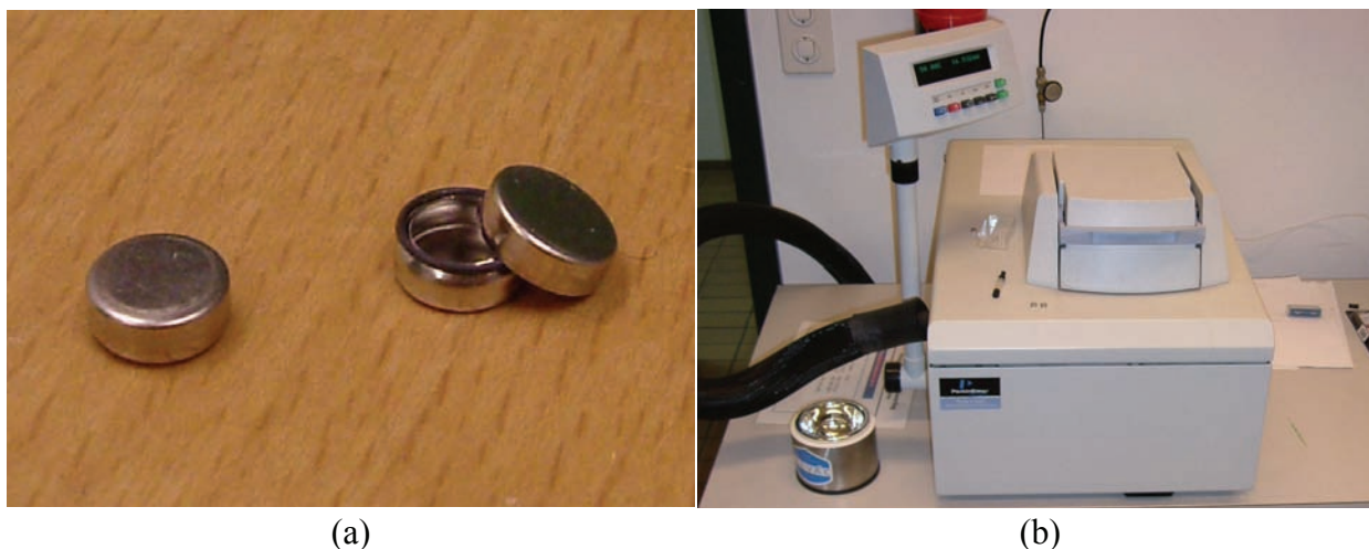
Figure 1.10: (a) Medium-pressure stainless steel crucibles consisting of bottom, cover and O-Ring, (b) Perkin-Elmer Pyris1 DSC with Intracooler
