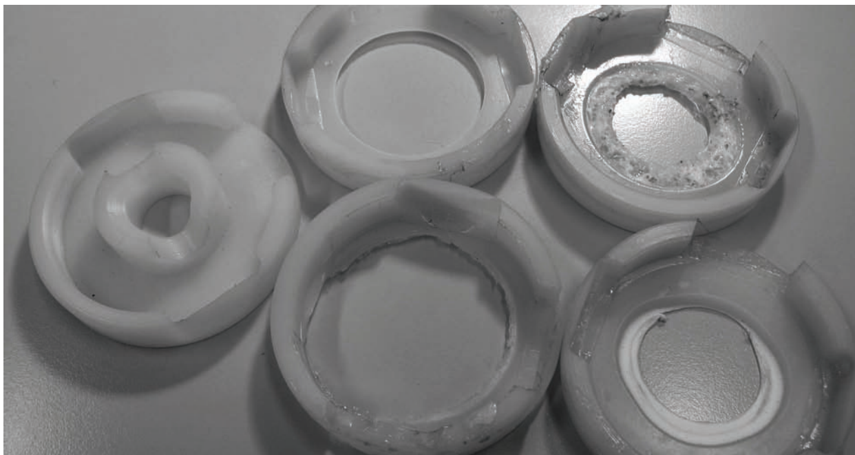
Figure 4.18: PVDF filling parts before (left) and after use. The material has been completely dissolved by the reaction media.
