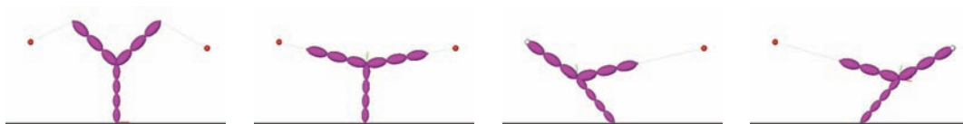
Figure 3.2: Comparison between weighting and priority strategies. Left: Initial configuration with conflicting tasks. Middle left: Solution using weighting strategy to solve conflicts. Middle right: Solution using priority strategy to solve conflicts (the left task has a higher priority than the right one). Right: Solution using priority strategy to solve conflicts (the left task has a lower priority than the right one).
