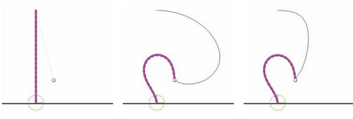
Figure 3.12: Paths followed by the end-effector depending on the IK method. Left: Initial configuration. Middle: Transpose of the Jacobian. Right: Damped least squares inverse of the Jacobian.
