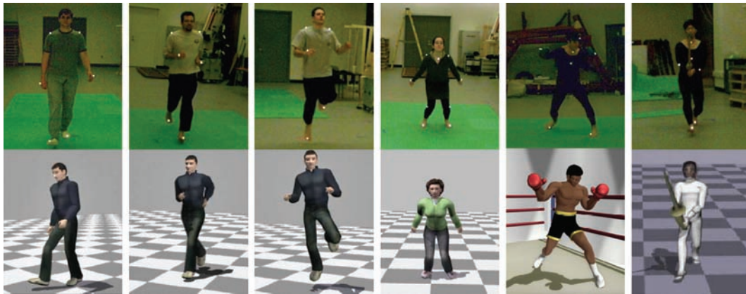
Figure 2.4: Users wearing a few retro-reflective markers control the full-body motion of avatars by acting out the motion in front of two synchronized cameras. From left to right: walking, running, hopping, jumping, boxing, and Kendo (source: [Chai and Hodgin, 2005]).
