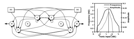
Fig. 2. Left: The neuronal oscillator. A black point indicates an inhibitory connection, a fork indicates an excitatory connection. The neurons of type B are not connected to any other neuron and can therefore be removed from the network. **Right**: Evolution of the frequency and amplitude when varying the input drive (BS). The vertical lines determine the region in which the amplitude and frequency increase monotonically.
