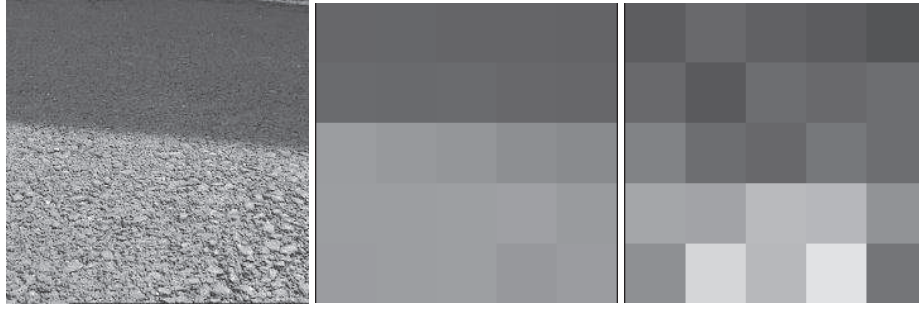
Figure 3: Left: Snapshot from the robot camera. Center: Pixel average. Right: Pixel sample.
