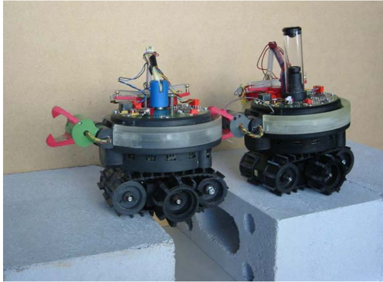
Figure 13. Swarm-bot prototype using the rigid connection to pass a gap.
