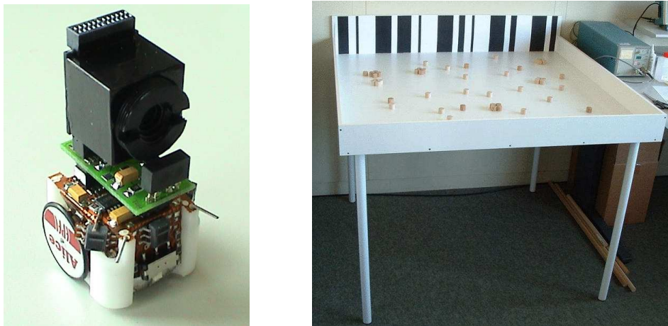
Figure 4. Left: The sugarcube robot Alice equipped with vision system, distance sensors, communication sensors, and two frontal „mandibles“ to better grasp objects. Right: The arena with small and large objects. The nest is under the textured wall where a small gap let objects –but not robots—fall on the floor.
