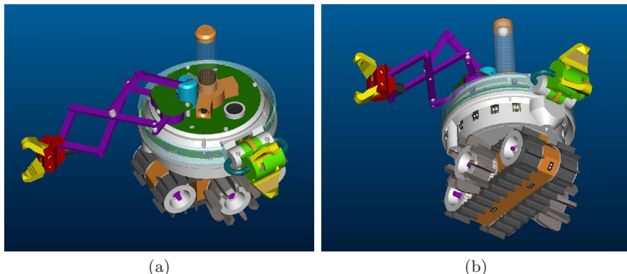
Fig. 2. Graphic visualisation of the s-bot concept. (a) The main body (turret), which has a diameter of 116 mm, is equipped with passive and active gripping facilities, sensors and electronics. (b) The lower body (traction system) is equipped with tracks and hosts the batteries.
