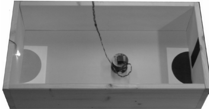
Figure 3: A mobile robot Khepera equipped with a vision module can gain fitness points by staying on the gray area only when the light is on. The light is normally off, but it can be switched on if the robot passes over the black area positioned on the other side of the arena. The robot can detect ambient light and wall color, but not the color of the floor.
