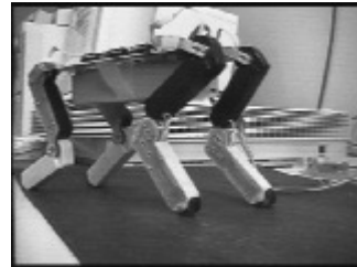
Figure 2: An evolved 4 legged robot. The control system of the robot, its body size, and length of legs have been evolved in realistic 3D simulations. The physical robot in the picture has been partially built according to the evolved genetic specifications. The evolved control system is transferred from the simulated to the physical robot. Such evolved robot can walk and avoid obstacles. The robot is approximately 20 cm long and weights less than 1 kg without batteries. Leg control is given by low consumption HC11 microcontrollers.
