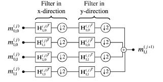
Fig. 2. Recursive computation of  $m_{1,1}^{(j+1)}$  using multichannel two-scale filters.
