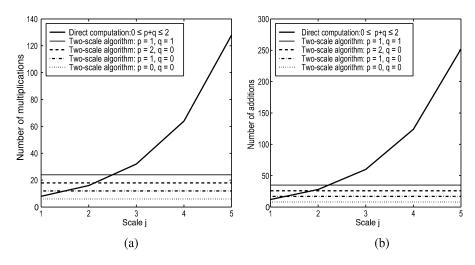
Fig. 13. 2-D computational complexity per output point for direct moment computation and usage of two-scale algorithm. (a) Number of multiplications. (b) Number of additions.
