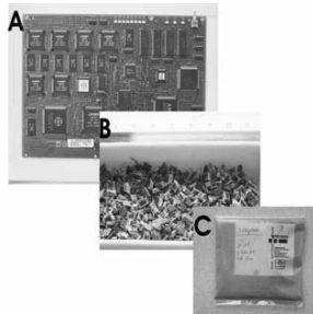
Fig. 6.1: PWBA before cutting (A), manually cut PWBA (B), pulverised PWBA (C).
