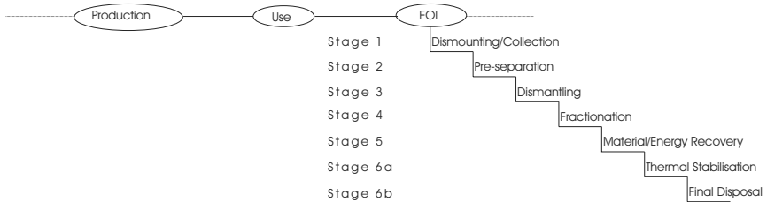
Fig. 2.3: Subdivision of the EOL phase of mobile phone networks into consecutive stages.
