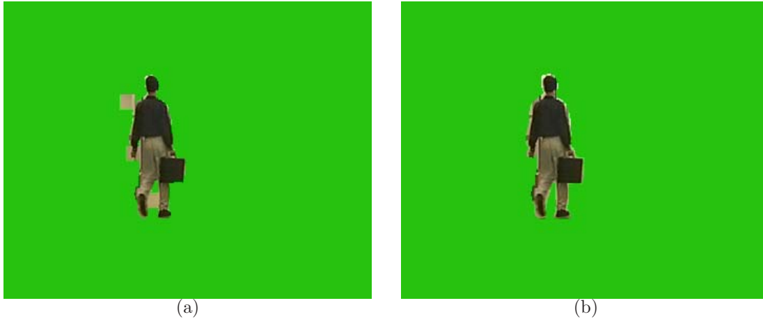
Figure 5.5: Example of border holes with the same amount but different distance from the ideal contour (a) large spatial errors (b) small spatial errors.
