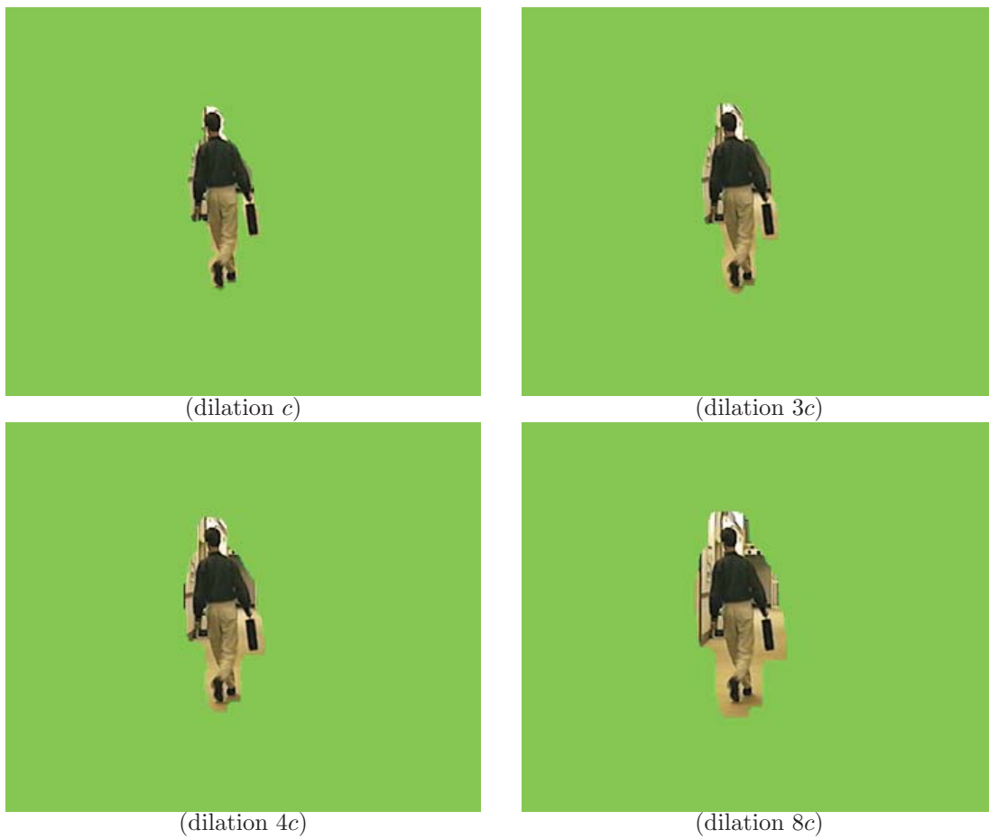
Figure A.2: Sample frames for different amount of the added background artifact ( c is equal to number of pixels on the contour object) for the video sequence “Hall monitor”.
