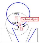
If we explicit the case of the spherical joint, we obtain the following torsor  $[\tau_{\text{spherical joint}}]_{\text{Osth}}$ (between Osr and Ocr), calculated at point Osth (Osth is the theoretical centre of the sphere, Osr is the real centre of the sphere, idem for the points Octh and Ocr characterising the cone):
