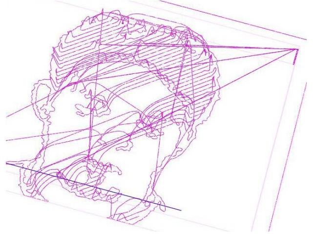
Fig. 8. 3D trajectory of the right hand in Cartesian space. The transitions between the strokes are depicted, as well as the trajectories used to refill the pen (the ink-pot position is on the top-right corner of the drawing).
