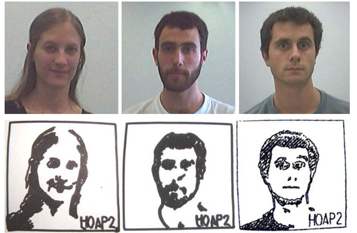
Fig. 10. Top : Faces detected from the webcam (subspaces \mathcal{R}_2 ). Bottom : Final portraits drawn by the robot, using different kinds of pen (marker pens and quill pen).
