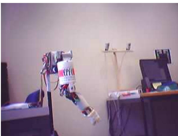
Figure 7: Photo of the 7DOF prototype of Robota arm taken by Robota eye camera
