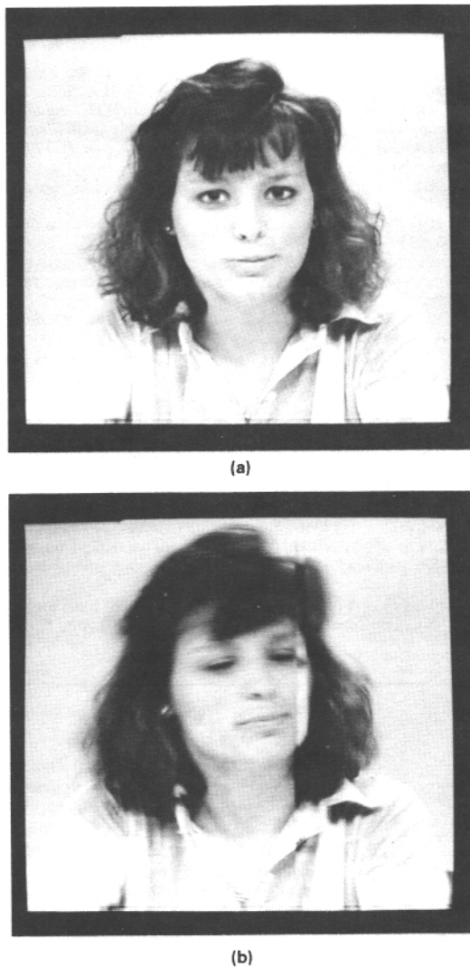
Fig. 16. Lossy transmission with one packet lost per frame in band 1 and five packets per frame in bands 2 through 11. Note that the lost data appear in different locations in (a) and (b).
