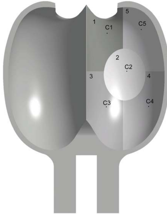
Figure 2 View of the 5 bucket zones (1 to 5) and the pressure probes locations (C1 to C5)
