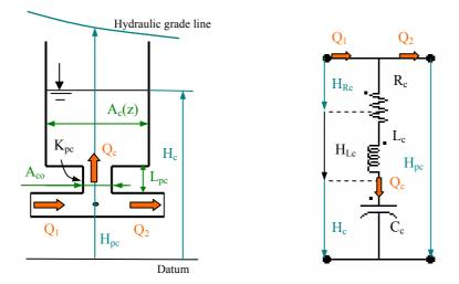
Fig. 3 Surge tank modelled using impedance method.
