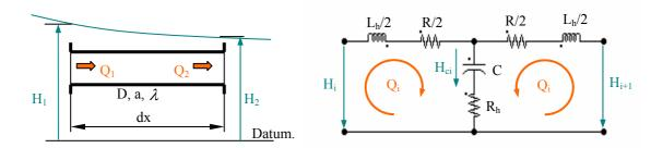
The Fig. 1 presents the impedance model for a pipe of length dx:
