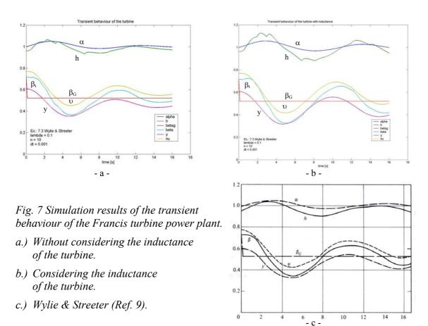
The 30% decrease of the rated torque  $\beta_G$  of the generator induces an increase of the rated speed  $\alpha$  which induces itself the reaction of the controller which commands the closure of the
