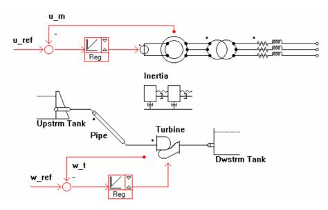
*Fig. 5 Modelling with SIMSEN of a power plant including a Francis turbine coupled to a generator.*
