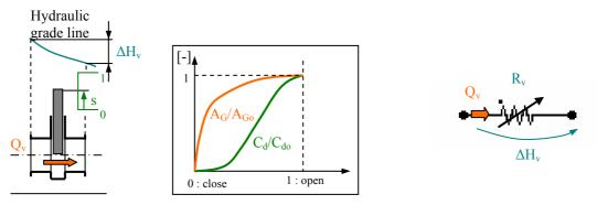
Fig. 2 Valve modelled using impedance method.
