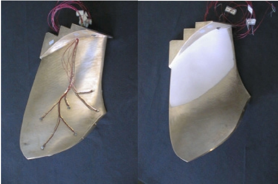
Figure 2: Photographs showing transducers mounted in the runner blade and the finished blade
