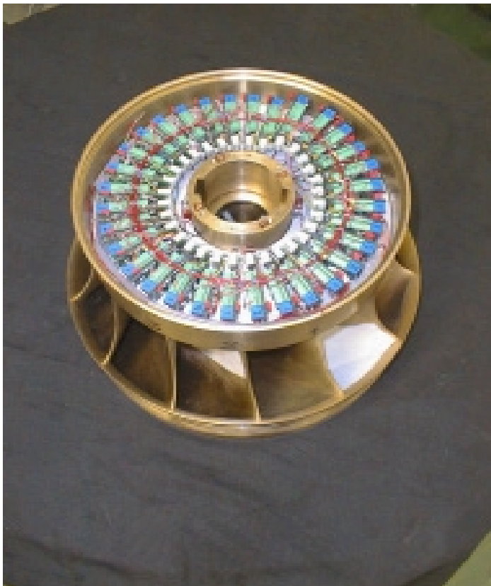
Figure 3: Photograph of the runner crown with data collecting modules
