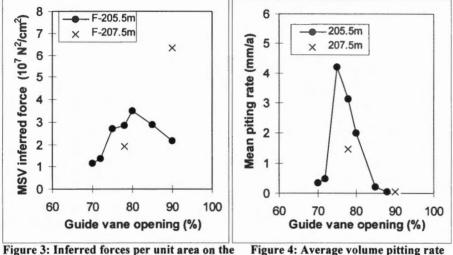
Figure 3: Inferred forces per unit area on the Figure 4: Average volume pitting rate proto (lower guide bearing acceleration) on 4 disks for same tests on the proto.
