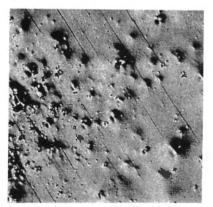
Figure1: typical pitting on the prototype on 316L SS (130 HB)
