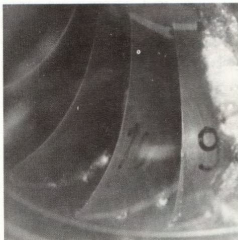
Figure 5-a Cavitation test at the plant cavitation number, the operating point corresponds to the full load and the nominal head ; \dot{V}/\dot{V}_A = 1.13 .
