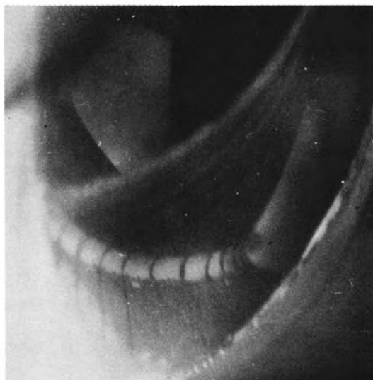
Figure 9: Photograph of inlet cavitation at the high head point H = 30 m \sigma = 0.08
