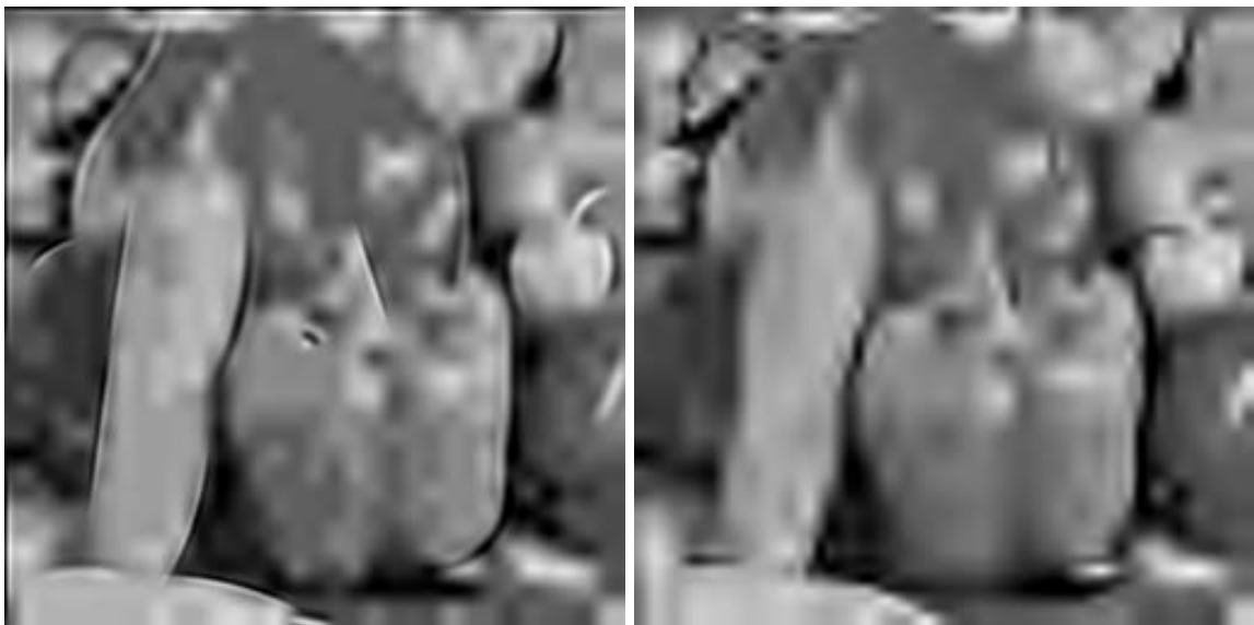
Figure 5.4: Comparison between JPEG2000 and MPW at about 0.05 bpp. Top: original peppers image ( 256 \times 256 ). Bottom left: image compressed with MPW (PSNR = 23.13). Bottom right: image compressed with JPEG2000 (PSNR = 21.36).
