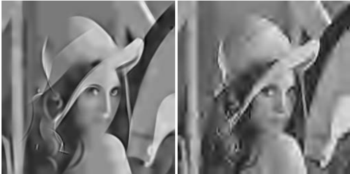
Figure 5.9: Comparison between JPEG2000 and the proposed scheme based on MP at 0.079 bpp for the image Lena of size 256 \times 256 . Left: image compressed with MP (PSNR = 25.51). Right: image compressed with JPEG2000 (PSNR = 24.32).
