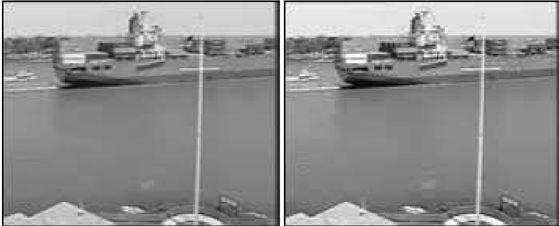
Figure 5.19: 16th frame of the sequence container in QCIF format coded with MP (left) and 8x8 DCT (right)
