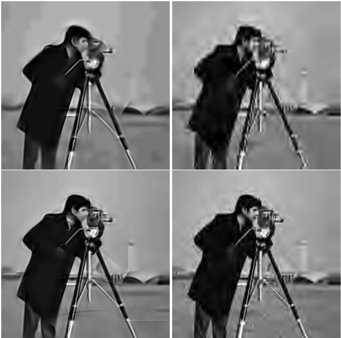
Figure 5.10: Comparison between JPEG2000 and the proposed scheme based on MP at 0.077 (top) and 0.147 (bottom) bpp. Top left: image compressed with MP at 0.077 bpp (PSNR = 23.92). Top right: image compressed with JPEG2000 at 0.077 bpp (PSNR = 22.62). Bottom left: image compressed with MP at 0.147 bpp (PSNR = 25.61). Bottom right: image compressed with JPEG2000 at 0.3 bpp (PSNR = 25.13). The original image can be seen on the top of Fig. 5.6
