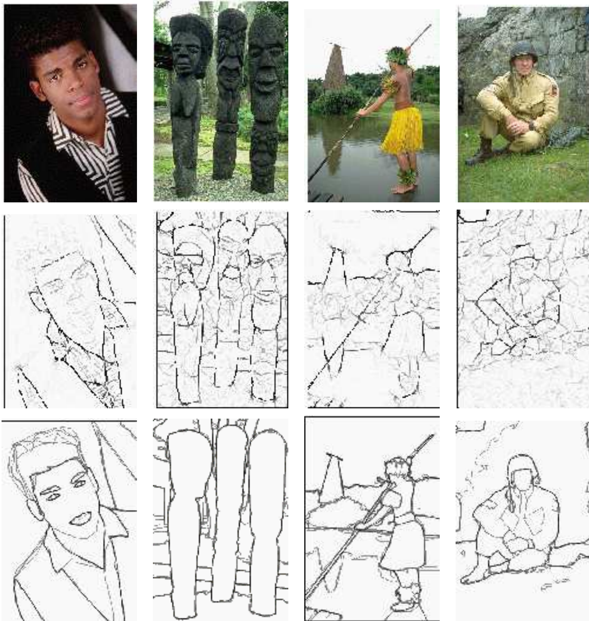
Figure 3.6: Results obtained by Martin et al. (2004) using the texture and brightness gradient cues (second row) of images shown in the top row. Human extracted edges are shown in the third row. Images courtesy of Martin et al. (2004).
