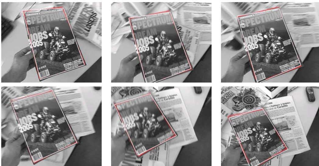
Figure 5.12: Tracking in motion blur using a classifier trained using the database composed of patches selected from Fig. 5.10. The fitted model is shown by the white wire frame.
