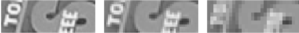
Figure 5.11: Magnified samples of the border of a magazine. The database for learning the borders of a specific object is made using small patches selected from borders of the object in three levels of resolution. These patches are then concatenated against random backgrounds to form the training data.
