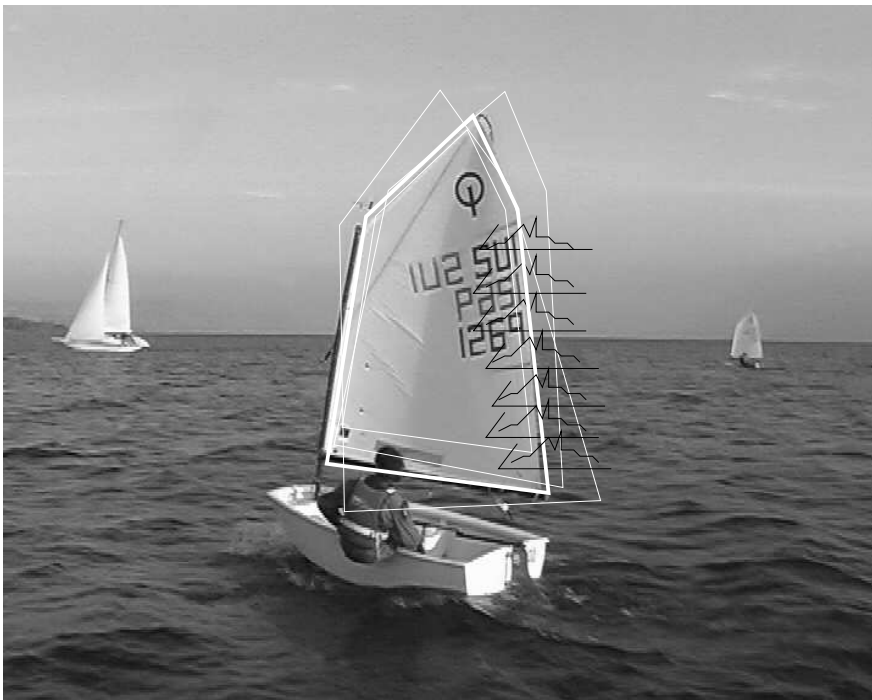
Figure 6.2: RANSAC fitting of the model. Some drawn hypotheses for the sail pose are shown. Some illustrative scanstripe probabilities which are used to calculate the support of each hypothesis are also depicted in black.
