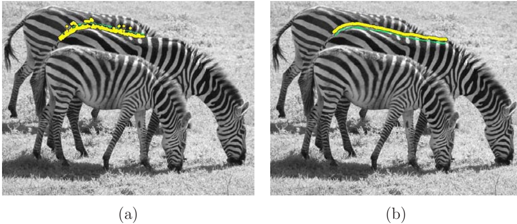
Figure 7.16: Boundary detected by Markov model and scanstripes corresponding to Fig. 7.15-(b). In (a) We use the Markov model technique on independent scanlines while in (b) we use the scanline results in conjunction with the Viterbi algorithm to extract a continuous boundary between the zebras.
