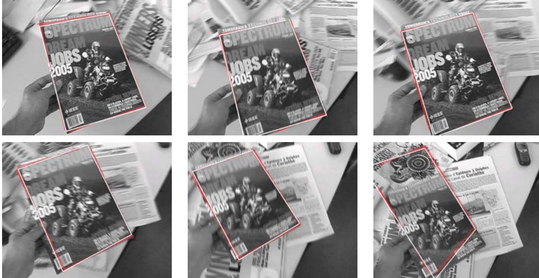
Figure 5.13: Tracking in motion blur using the classifier trained using a database composed of general texture boundaries as explained in Section 5.2. The fitted model is shown by the white wire frame.
