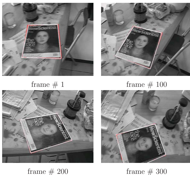
Figure 8.14: Tracking with KLD-based update of the prior model. RANSAC is used to fit straight lines (shown in red) to the scanstripe probabilities directly which are then used to calculate the pose of the model (white wire frame).
