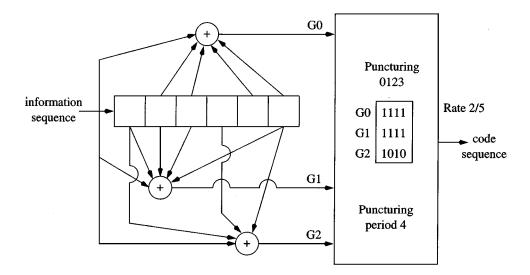
Fig. 20. Convolutional code notations. Rate-1/3, memory M = 6 mother code with puncturing period P = 4. The output code rate is 2/5.
