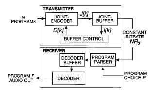
Fig. 12. The joint encoder is treated as a single encoder. The bitstream parser at the receiver extracts the bitstream of a specific radio program P.
