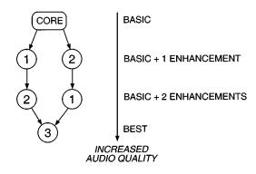
Fig. 15. The core bitstream can be enhanced in different ways for better audio quality: embedded audio coding.
