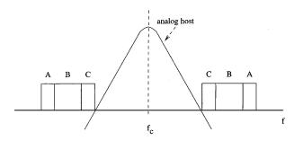
**Fig. 19.** Basic hybrid IBOC concept. Bands A–C of the OFDM carriers have different interference susceptibilities, and this impacts the channel code design. Band A is more sensitive to interference than band B. Band C is used optionally.
