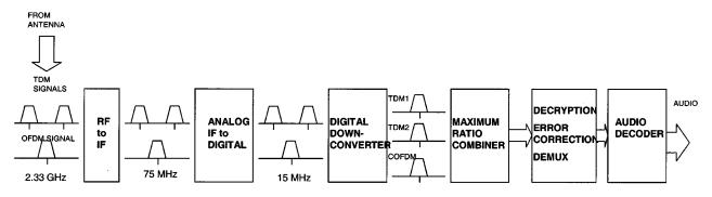
Fig. 30. Decomposition of SDARS receiver chip set.
