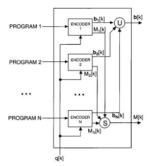
Fig. 11. The bitstreams of the N encoders are combined. The bit rate of a joint frame is J[k]. A single common distortion criterion is used.
