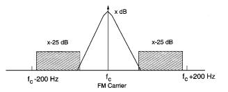
Fig. 18. Basic FM power spectrum.
