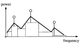
**Fig. 5.** The spectral coefficients are divided into coding bands. Each coding band is quantized such that the error is just below the masked threshold.
