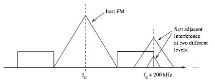
Fig. 21. Impact of a first adjacent FM interference signal at  $f_c$ +200 kHz at two different levels. Alternatively, the first adjacent interference may appear at  $f_c$ -200 kHz.
