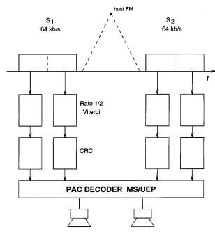
**Fig. 22.** Simplified block diagram for a proposed system based on 64-kb/s multidescriptive PAC and two-level UEP. The multistream transmission is done for four streams and the interleavers are not shown explicitly.
