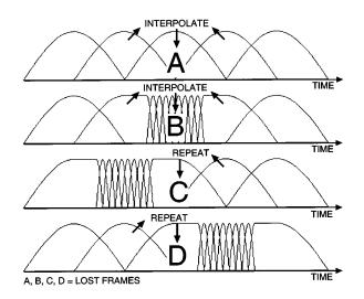
Fig. 13. An example of four different cases for mitigating a lost frame.
