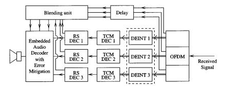
Fig. 25. Receiver for multistream transmission. Conceptual diagram. The OFDM demodulator also contains synchronization, training, equalization, and timing.
