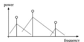
Fig. 4. The masked threshold is computed by considering the masking effect of each spectral component of the audio signal.
