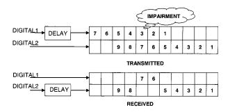
**Fig. 28.** Concept of time diversity. By delaying stream 1 during transmission, the receiver has two versions available. The contents will be impaired at different time instants.
