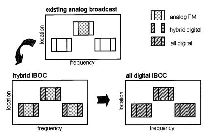
Fig. 17. IBOC transition from analog to digital.
