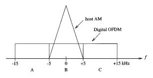
**Fig. 23.** Conceptual power spectrum of a 30-kHz, hybrid 1130C-AM. The digital data is transmitted in bands A-C.
