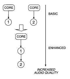
Fig. 16. Multistream audio coding: two independent bitstreams combined yield a bitstream with enhanced quality.
