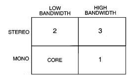
**Fig. 14.** The core bitstream provides basic audio quality. Bitstreams 1–3 enhance the audio quality.
