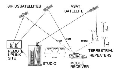
Fig. 27. Basic SDARS system. This configuration matches the Sirius Satellite Radio system.
