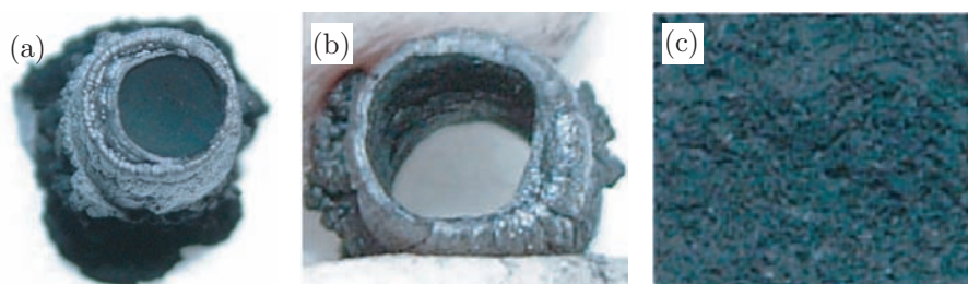
Figure 3.2: (a) the arc-discharge product (b) hard shell (c) soft core.
