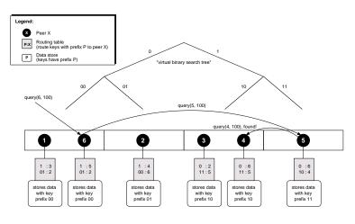
Fig. 1. Example P-Grid
