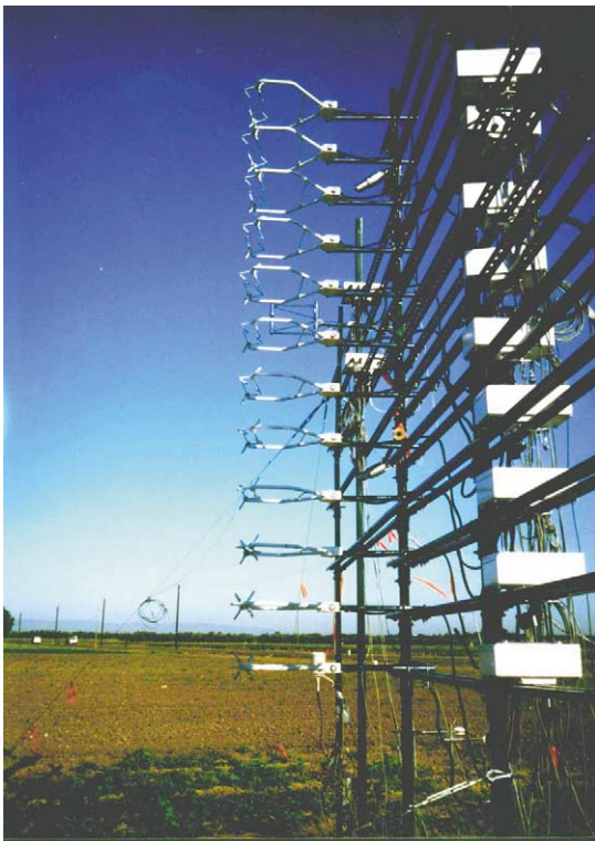
Fig. 6. Photograph showing the vertical array of 3D sonic anemometers.
