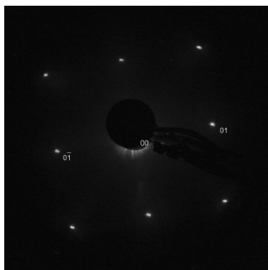
Figure 2.20: LEED pattern of a clean Ni(100) acquired using an electron beam energy of 103 eV (picture from Schmid Ph.D. thesis 71 ).
