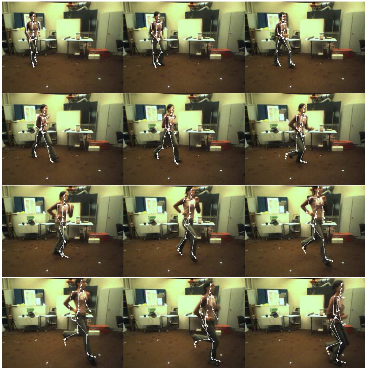
Figure 10: Tracking the transition between walking and running. In the first four frames the subject is running. The transition occurs in the following three frames and the sequence ends with running. The whole sequence is shown. Corresponding movies are submitted as supplementary material.
