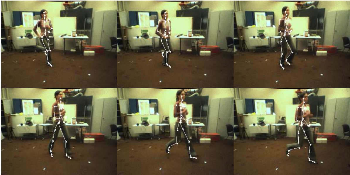
Figure 7: Tracking a running motion assuming a constant style. The legs are correctly positioned except the left one in the first frame. Movies are submitted as supplementary material.
