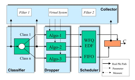
Figure 2: General block diagram of packet processing modules within a router
