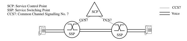
Fig. 1. Simplified architecture of the Intelligent Network.
