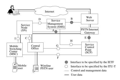
Fig. 7. Reference Model for PSTN/Internet Interworking (PINT) (augmented from [24])
