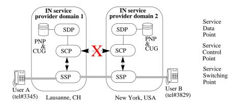
Fig. 9. Provision of a VPN service across two IN provider domains
