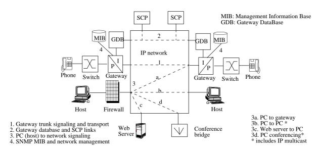
Fig. 11. A standards framework for IP telephony [39]
