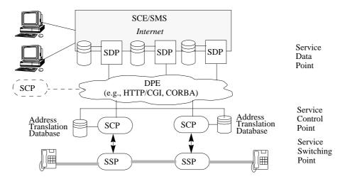
Fig. 8. The WebIN physical architecture (adapted from [36])
