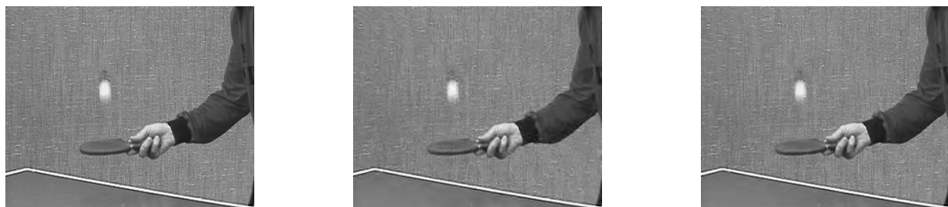
Figure 3.22: Visual comparison between both versions of the 25th frame of the first GOP of the table tennis sequence (left: original frame, middle: non-adaptive, right: adaptive). This example illustrates how in the most evident cases, the contours of moving objects are better preserved when adaptivity is in use. Ringing is lighter around areas nearby contours.
