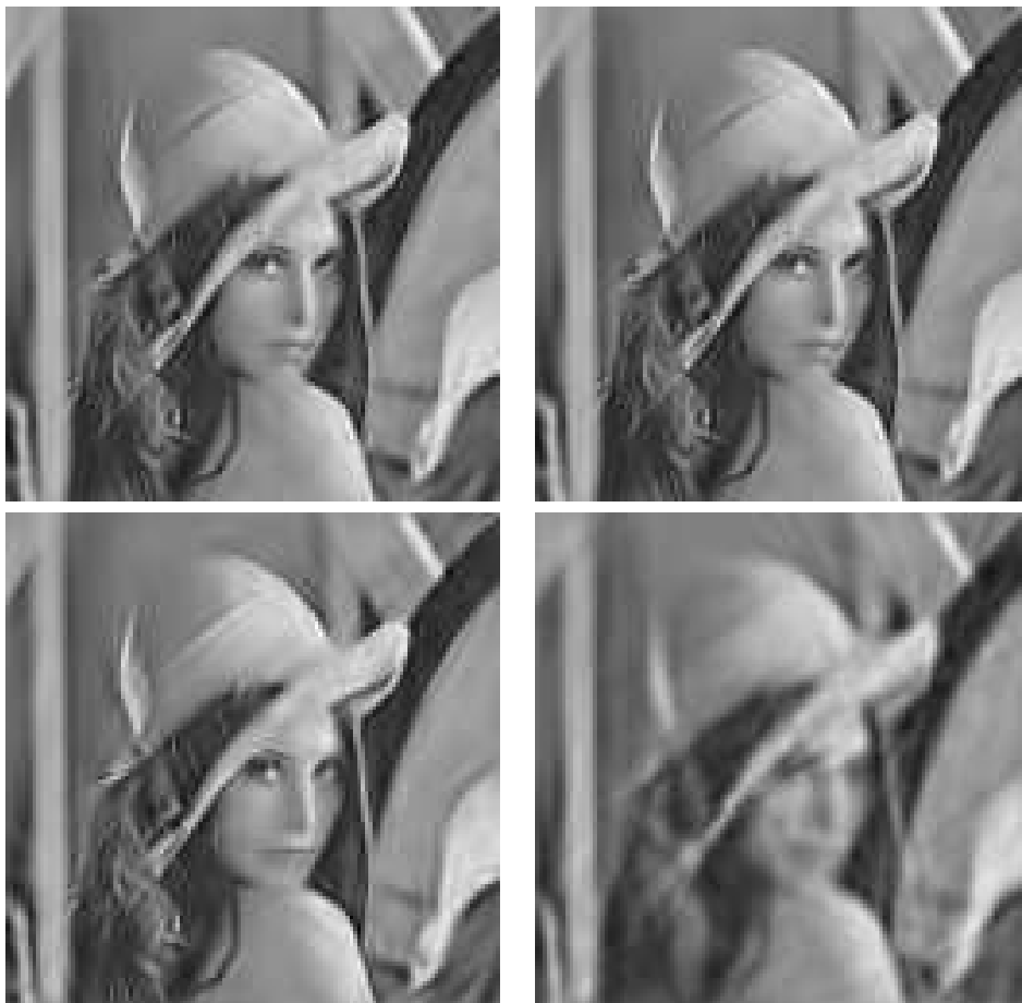
Figure 6.15: Visual comparison of the different approximation of Lenna 128x128 for the amounts of memory of: (from left to right and then up/down) 377 MB (threshold 0), 122 MB (threshold 10^{-4} ), 22 MB (threshold 1) and 2.2 MB (threshold 10).
