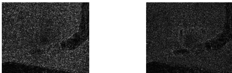
Figure 3.23: Visual comparison between the absolute value of the residual error after compression of the 25th frame of the Table tennis sequence. On the left, we see the residual signal that corresponds to the fixed decomposition structure and compression rate of 804.2 kbps. On the right, the residual generated by the adaptive scheme at 781.98 kbps can be seen.
