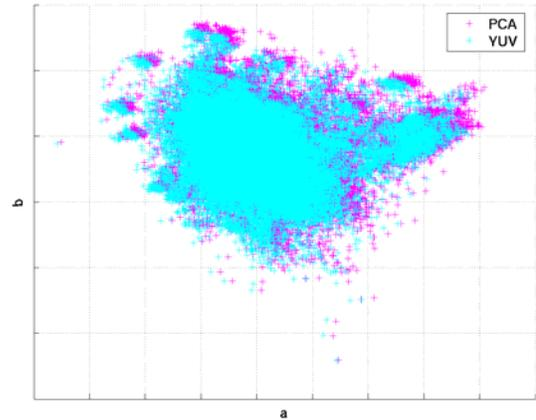
Figure 6. Plot of the a, b chromaticities of the two images of Figure 5. The image treated using  $f_{YUV}$  is plotted in cyan while the image treated using  $f_{PCA}$  is plotted in magenta.
