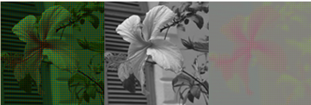
Figure 4: (a) Mosaiced color image according to the Bayer CFA, decomposed as (b) luminance plus (c) sub-sampled opponent chromatic channels.
