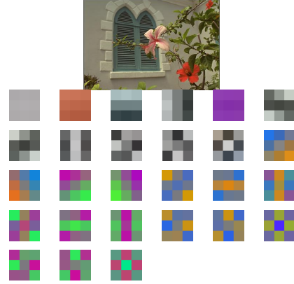
Figure 2: (a) Image (b) Spatio-chromatic representations of eigenvectors of the covariance matrix (with V = 3 ). Vectors are arranged in rows of decreasing eigenvalue magnitude.
