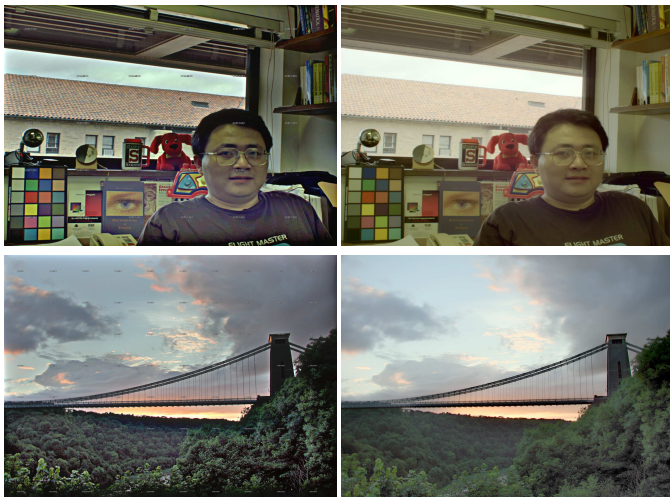
Fig. 9. Left: Image treated with MSRCR. Right: Image treated with the adaptive filter method.
