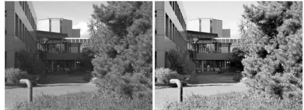
Fig. 1. Example of HDR scene that requires local processing. Left: Image rendered using a gamma correction. Right: Image rendered with the Retinex-based adaptive filter proposed in this article that combines global compression and local processing.
