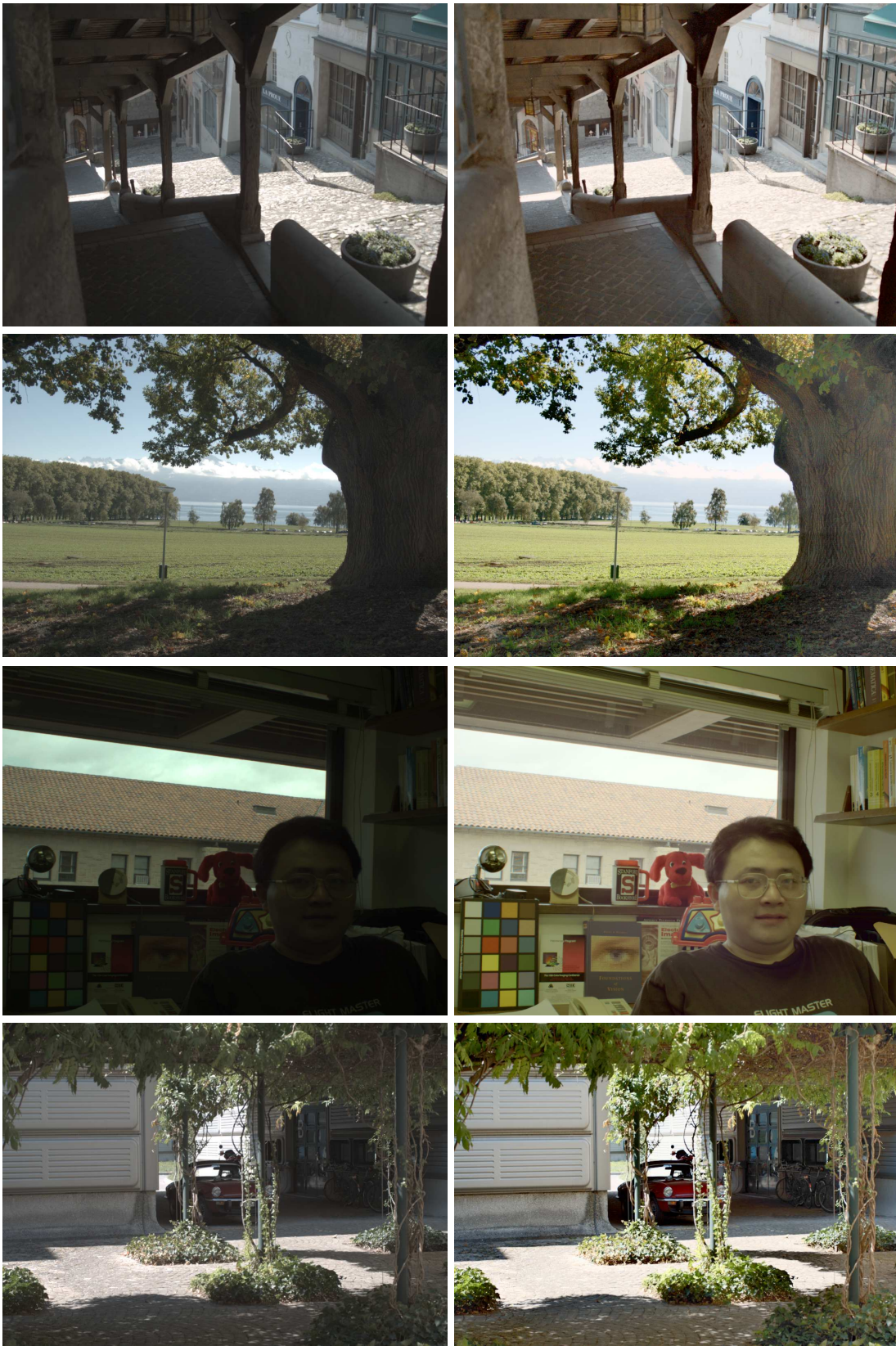
Fig. 12. Results of the Retinex-based adaptive filter method. Left: Gamma-encoded image. Right: Image treated with our method.
