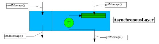
The Asynchronous Layer has its own thread, which will always try to get the next message from the layer below, using the method getNetwork Message(). If no message is available, the lower layer's getMessage() method will block until a new
