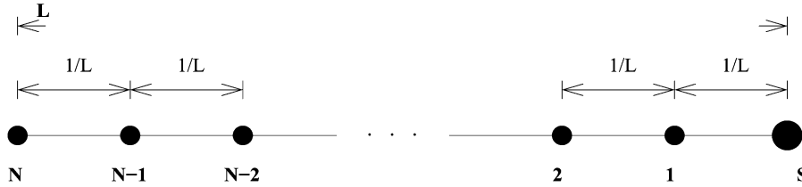
Fig. 2. A 1-D grid with constraint on the total distortion. Nodes are labeled with increasing indexes, with node 1 closest to the sink and node N farthest. The correlation model is \exp(-ad_{i,j}) . (a) Distortion allocation as a function of node index. (b) Rate allocation as a function of node index.
