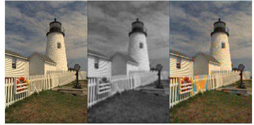
Figure 4: Left: original image. Center: luminance image. Right: reconstructed image, the luminance estimated with the filter of equation (4).
